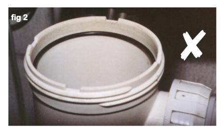
DO NOT assemble heater with 'O' ring as shown. This will dislodge when head and body are engaged causing water damage to the electronics. However, lightly lubricating the inside of this lip is permissible and will assist in assembly.
