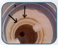
Remove any existing tabs with chisel/hammer and/or pliers.
