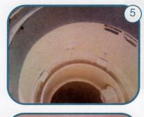
Test fit ring with Twedge. Place ring in canister so wedge notch is on side without a port. The ring feet must sit between the canister wall and the lid seal ring so the ring is level. The ring must tighten in canister at or before bottoming the T-wedge into the notch. The Twedge must be placed in the ring so the step is toward the inside. Incorrect placement could cause interference between the ring and internal lid.
