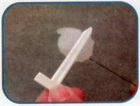
Place the ring into position and then quickly wipe the T-wedge on the glue dauber and fully insert it into the ring notch and ensure that the ring is level.
